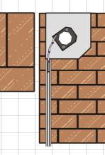
In Built system allows the shutter box to be hidden completely when viewed from the building exterior.
